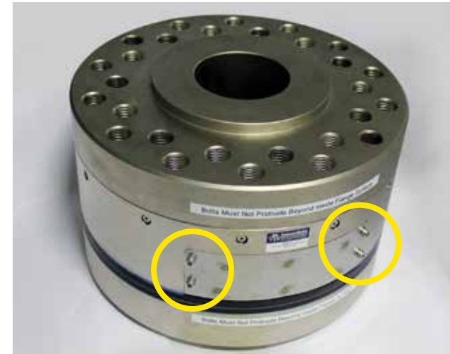
1: Battery module access: Batteries are located inside sensor behind the module access panel. Remove the (4) 1/4-28 socket head screws located on the corners of the battery module.
