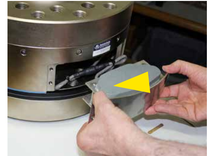
2: Carefully remove battery module: Grasp battery module firmly by the corners and pull out.
