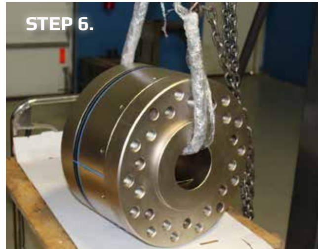
Place sensor on clean, flat work surface: Be sure to place sensor with battery panel facing up.
