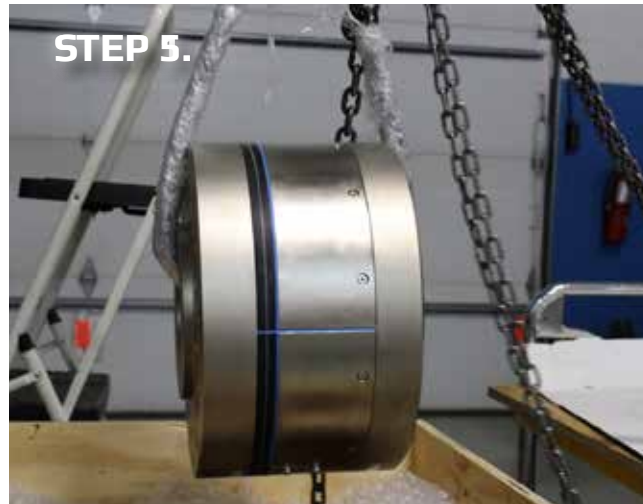
Slide chains through sensor: Make sure chains have a protective surface around sensor. Lift with hoist.
